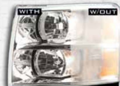
Half of this headlight was protected with Husky Shield Headlight Guard and sand blasted at a distance of 12"
