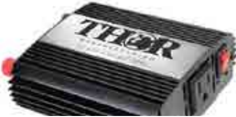
TH225 Modified Sine Wave Inverters • Continuous output power: 225 Watts • Surge power capability (peak power): 450 Watts • DC input / operating voltage: 11 to 15 Volts • Output voltage: 120 Volts ac / Output frequency: 60 Hz / Output wave form: modified sine wave PN: THOTH225
